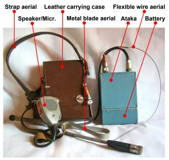
Ataka in a leather carrying case with aerials and combined speaker-microphone. The latter had a channel switch, volume control with on/off switch, PTT button, and two tone buttons.
