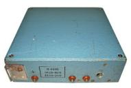
Bottom view of Ataka showing battery contacts and fixing arrangements. The set had a die-cast aluminium alloy frame.
